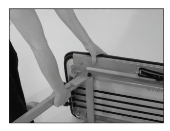
Turn the carriage upside down so it is cord side up. Using a crescent wrench and flat head screwdriver, remove the screw that is holding the wheel in place. Replace the old wheel with the new one, add the washer, push the screw through the wheel and tighten with the nut.
