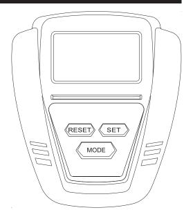
**RESET :** In the setting mode, press the button to reset the setting values to zero.
