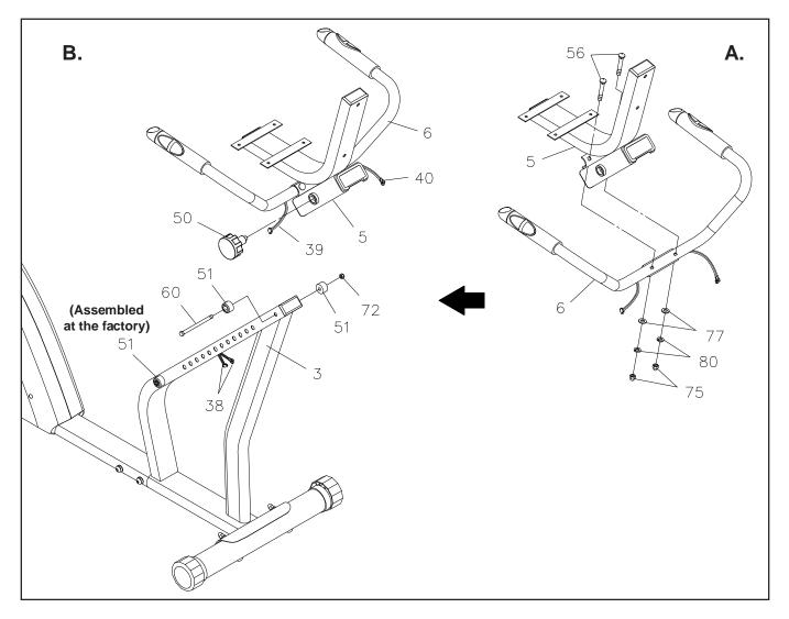
NOTE: Be careful not to damage the WIRES(38, 39, and 40) when attaching the HANDRAIL(6) and the SEAT FRAME(5).
